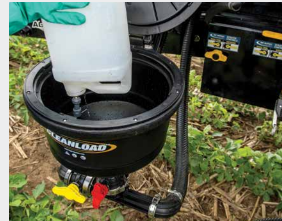
Cleanload System Is A Self-Contained Inductor System Which Allows The Operator To Mix Liquid And Dry Chemicals Safely And Quickly.
