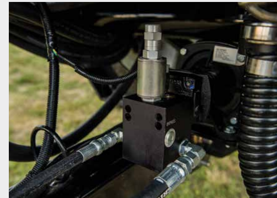
Hydro Cast Iron Pump (210 GPM) With Pwm Valve Allows Greater Variation In Speed.
