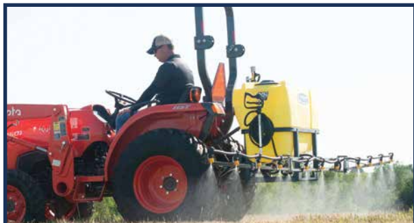
Spraygun holder and 25' hose wrap can be mounted on either side of the unit. Conveniently mounted for easy operator access.
